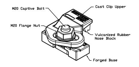
The Atlantic Track F1-37 Adjustable Crane Rail Clip is designed specifically to fix Crane Rail mounted on a narrow support beam or plate.
