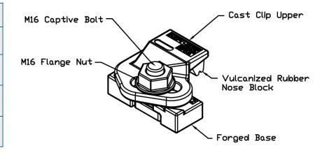
The Atlantic Track F1-27 Adjustable Crane Rail Clip is designed specifically to fix Crane Rail mounted on a narrow support beam or plate.
